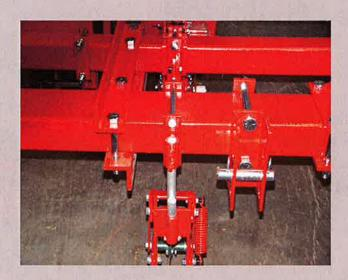
5. Mount the swivel coulter to the 4x7 toolbar so that it lines up with the center of the No-till tooth.
