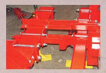
3. At the row centers, mount the No-till bracket to the 4x4 toolbar. If this is for a 5000 series transplanter, the unit hitch must also be mounted with the No-till bracket.
