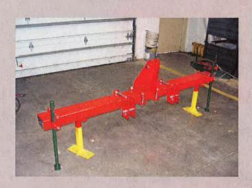
1. Mount the 3-point hitch and the pipe stands to the 4x7 toolbar.
