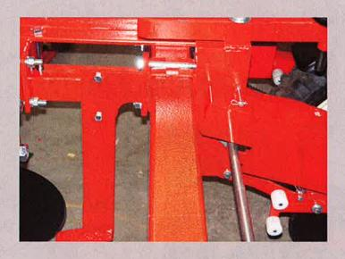
4. Attach the No-till tooth to the bracket.
