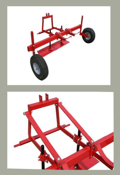
7. Tip front assembly upright so it stands on leveling blade and the gauge wheels.
