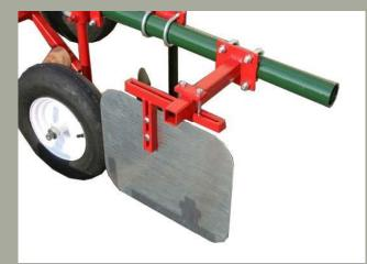
18. Finished Model 90 set up for 4' plastic. Shown with optional DRIP EXT attachment.
