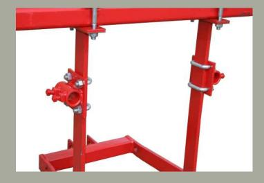
2. Use four FUB1221 U-bolts to fasten leveling blade brackets to 3-Point side arms. Leave U-bolts slightly loose until shanks are inserted in step 4.
