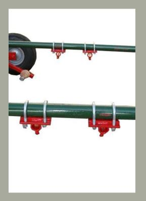
15. Use two 7/8" set collars to mount each smooth wheel to axle. Tilt front shank clamps and slide wheel shanks into pipe. Tighten these clamps 29" from toolbar to front edge of clamps. Set wheels on slight angle with shank straight down with about 5" of shank showing above clamp. Tighten set screws.  Take the four shank clamps and put two #9034 U-Bolts on each clamp. Slide two clamps onto each side arm. Leave loose.
