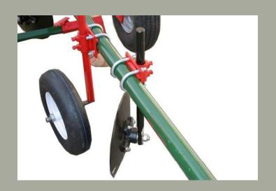
16. Tilt the back shank clamps and slide rear coulter into clamps. Angle coulters out. Tighten clamps 40" from toolbar to front edge of clamps. Tighten set screws with 4-1/2" of shank showing above clamps.
