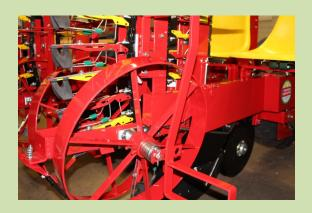
13) Install the plant stand by removing the outer cotter key on the axel. Place over the top of the wheel, then feed it onto the axel. Secure with two 3/8 x 1 bolts and flange nuts. Replace cotter pin.
