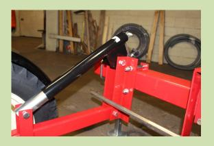
10) Install gauge wheel by using four 5/8 x 6 1/2 hex head bolts, nuts and washers. Use one 1/2 x 2 x 6" red securing plate.
