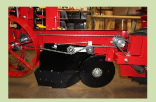
9) Install the unit drive chain to the drive. 146 pin (linked) \* Note—you need to add six links when installing the 24 tooth sprocket which is included in kit.
