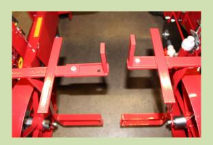
14) Install the outer plant box supports.
