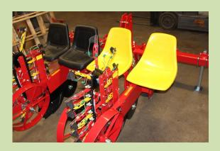
11) Install seats shown here with standard fiberglass and optional cushion with one 1 1/2 carriage bolt, flat washer and 1/2" crown hex lock nuts.
