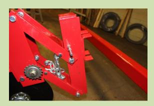
2) Remove he unit clamps from the unit and mount by using a 3/4 wrench and socket and secure the clamps by using two 5/8 x 6 1/2 hex head bolts, lock washers, nuts and two red securing plates. (1/2 x 2 x 6)
