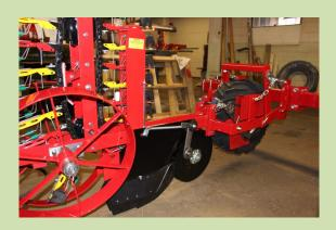
5) While supporting the drive, install the unit by using four 1/2 x 1 1/2 head bolts and nuts. Repeat with existing units.
