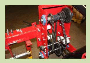
8) Install drive onto toolbar, align wheel with mark on the bar. Use four 5/8 x 6 1/2 bolts, nuts and washers. Use one 1/2 x 2 x 6" red securing plate.
