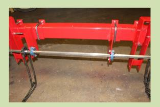
5) Install the shaft into the bearing plates. Replace hex head bolts, nuts and washers. Leave loose.
