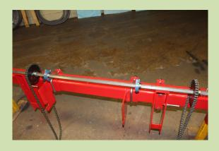
4) Remove the bearings and load the hex shaft with the bearing sprocket chains and shaft adaptor. 185 pin for 1100.
