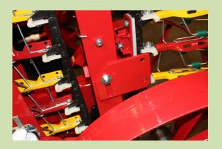
12) Install plant stand mounting plate by using one  $3/8 \times 1$  hex head bolt, one flat washer and nut. Leave loose.
