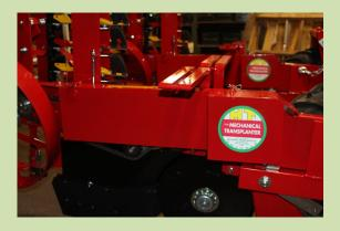
10) Install the outside chain guard by using two B-17 clip pins.
