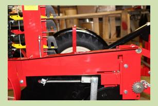
13) Install the unit inside chain guard if not already installed.
