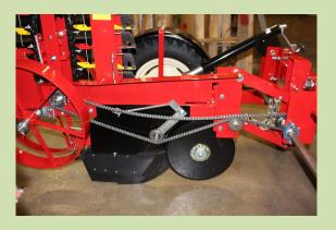
14) Install chain as shown. Align sprocket on the hex shaft and tighten. Set screw on the sprocket.
