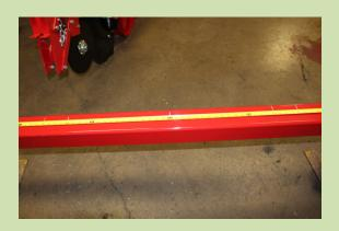
1) Set up your toolbar by marking your center (ie8' bar would be 48" or 4' center) mark you're a-frame drops 16" off center for cat II, 12" off center for CAT I. A) Mark your row center here. We are showing a standard 40" center. By marking 20" off center. B) Mark your drive centers here, we are showing a 80" by marking 30" off center.
