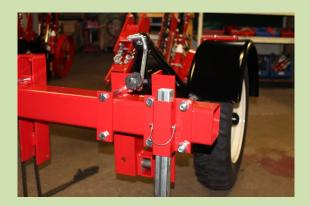
6) Install the pipe stands by using one 5/8 U-bolt , FUB 5844 nuts and lock washers . The other side of the brackets will be shared with the drive and gauge wheel held on by two 5/8 x 6 1/2 hex head bolts, nuts and washers.
