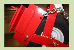
3) Install the unit clamps onto the drive ( these can be mounted with the angle iron facing out or in depending on space of the toolbar.) By using two #43 bushings,  $1/2 \times 1 \cdot 1/2$  hex head bolts, nuts,  $7/16 \times 1 \cdot 1/4$  flat washer and nuts. The TOP holes of the plates.
