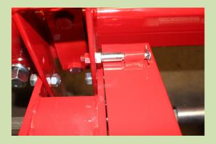
17) Install the last chain guard secure by placing one guard spacer and clip pin.
