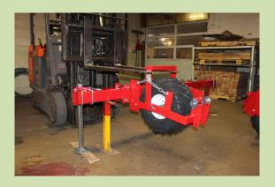
4) Install one drive system on the toolbar by using four 3/4 x 6" bolts for a 4x4 bar or a 3/4 x 9" bolts for a 4x7 bar, along with 4 nuts and lock washers. \* Note—the center tire will line up on your row center mark.
