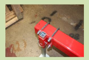
2) Install pipe stands for stability by using two FUB 5844 U-bolts, lock washers and nuts. Must be mounted opposite side of aframe to prevent the units from collaps-
