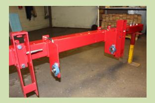
3) Install the two bearing plates by using one 5/8 U-bolt (5844) 1 red securing plate, nuts and lock washers.
