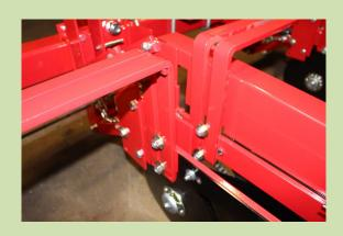
15) Install the red seat brackets by using one UB727 U-bolt, two flat washers and nuts. \* Note—when installing brackets on unit equipment with a double disc shoe attachments the brackets will be staggered.
