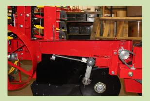
7) Install the inside chain guard by using one  $3/8 \times 1 \cdot 1/4$  hex head mold, flat washer and two nuts.
