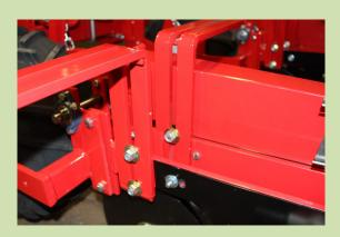
8) Install the red seat bracket "L" by using one UB727, two flat washers and two hex crown lock nuts.
