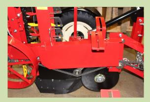
16) Install the outside chain guard secure with two B-17 clip pins.
