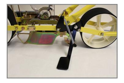
2) Install kickstand mounting plate with the slotted hole toward the front of the seeder. (see pic) Using the provided 8x22 mm bolt in the slotted hole and the re-used bolt in the round rear hole.
