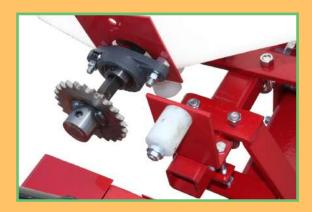
16. Set chain tightener bracket on end of small toolbar by drive side. Use two 3/8 x 3" bolts and 3/16 x 1-1/2 x 3-1/2" securing plate. Leave this bracket loose. Fasten plastic chain tightener to bracket using 3/8 x 3" carriage bolt. Center plastic tightener between sprockets so it is centered. Tighten bracket.
