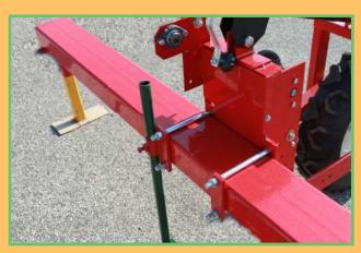
4. First, insert green pipe stand into mounting plate. Snug pipe so it is shorter than the stand under the toolbar. Slide 5/8 x 9-1/2" bolts in lower holes on drive. Put pipe stand plate against toolbar and secure with 1/2" nuts and lock washers. Now use 1/2 x 6" plate on other side and tighten nuts
