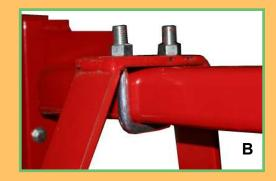
9. Use two UB1222 U-bolts on each toolbar. Lift toolbar up and push U-bolt in from bottom and secure with 1/2" nuts. Leave 5" of short toolbar showing on end next to drive wheel assembly. Center stands and short toolbars over row center marks. Tighten stands and toolbars.
