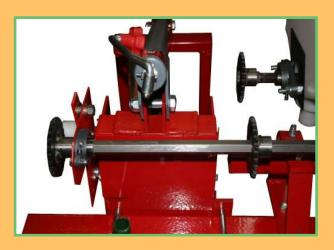
15. Tighten bearings and allen head set screws.
