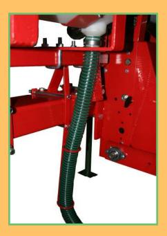
24. Slide hoses into holding brackets. Fasten holding brackets to toolbar using two 1/2 x 8" bolts and 3/16 x 1" x 6" securing brackets. Use upper or lower holes depending on how high the toolbar is run off the ground.
