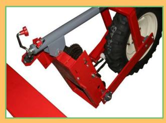
2. Take large guard off drive assembly so bolts can be inserted through inside holes
