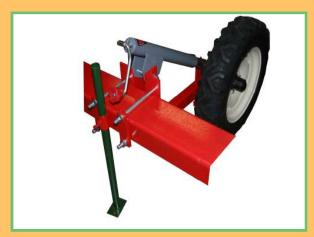
5. First, put pipe stand in bracket, then bolt gauge wheel assembly to toolbar by centering tire on wheel center mark. Use four 5/8 x 9-1/2" bolts, nuts, lock washers, pipe stand plate and standard 1/2 x 6" plate. Place pipe stand on outside bolts.
