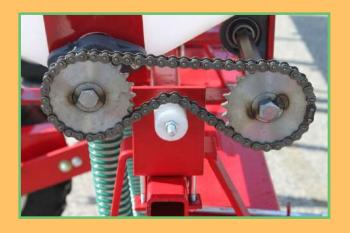
17. Install #40 x 61 link chain between hopper and drive shaft. Tighten chain tightener by sliding it up so chain is snug. Align sprockets and tighen set screws. Slide 3/8" washer onto chain tightener bolt.
