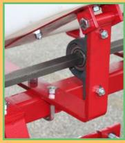
13. Loosen bearing on drive as shown. Loosen socket set screws in both bearings. Now slide hex shaft into first bearing. Place a 25 tooth sprocket on end of shaft between bearings. Slide hex shaft throught second bearing on hopper mounting bracket. Leave 2" of shaft showing on outside of drive side bearing.
