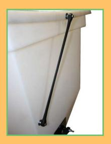
25. Fasten cover straps to hopper using four 1/4 x 1-1/2" bolts, six 1/4 washers and eight 1/4 flange nuts. Attach straps to hopper and top with the top off so straps are not stretched tight. Slide rubber strap through bolt, then flange nut (backwards) then washer. Insert into hopper. Use another washer inside hopper and secure with flange nut. On top only use washer on outside none on inside.
