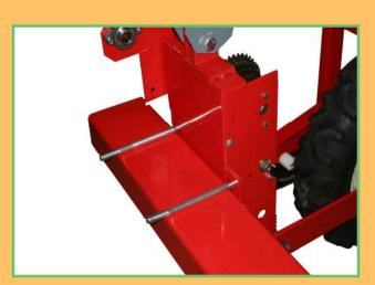
3. Put two 5/8 x 9-1/2" bolts through top two holes of drive mounting plates. Place drive on toolbar resting on the two bolts as shown.
