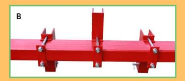
For CAT I, mark 13" off toolbar center mark and for CAT II, 16" Fasten lower arms to toolbar with two 3/4 x 9-1/2" bolts, lockwashers, 3/4" nuts and one 1/2 x 2-1/2 x 7" securing plate on each side. (Photo B)
