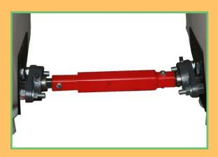
12. Install connector tubing between hoppers. Use 1/4 x 1-1/2 bolts and lock nuts. The connector sent is for 48" rows. For anything closer you'll need to cut large or outside tubing. Measure distance between hoppers. Allow 1/2" from each bearing when measuring. Hopper U-bolts must be really loose so you can tilt hopper backward or forward to put connector on shafts. Make sure holes on tubing connector ends are 90 degrees opposite each other. NOW tighten hopper U-bolts.
