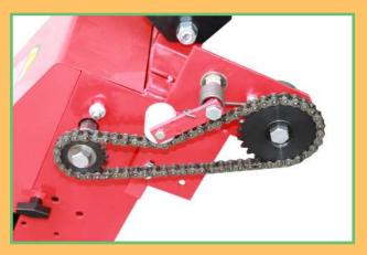
19. Use #40 x 62 link chain between upper drive sprocket and lower drive sprocket. Set plastic chain tightener against chain and tighten. Be sure that the tightener spring is set like the photo.
