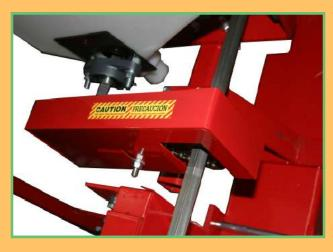
18. Slide chain guard onto bolt and tighten using 3/8" washer and jam nut on outside.
