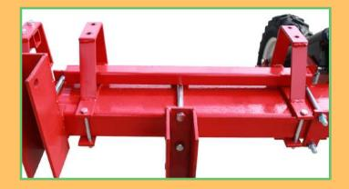
8. Lay a 2 x 2 x 3' toolbar under or inside each pair of hopper stands as shown.
