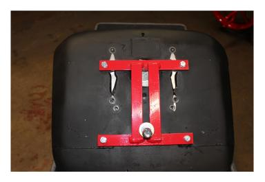
10) Install the red seat bracket onto the seat bracket if not already installed by inserting the  $\frac{1}{2}$  x 1  $\frac{1}{2}$  carriage bolt into the bracket. Use one flat washer, lock washer and hex nut to secure.
