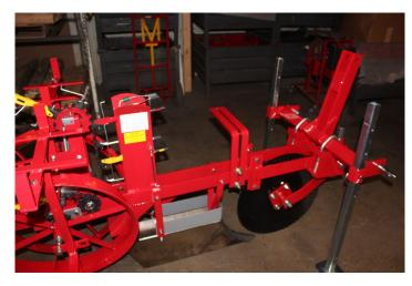
9) Install the red seat "L" bracket by using one #727 U-bolt, two flat washers, lock washers and nuts.
