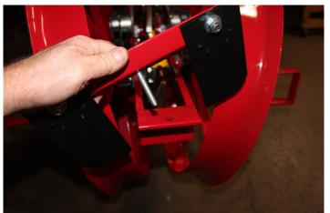
12) Install the rear weight bracket by removing the wheel scraper assembly.
