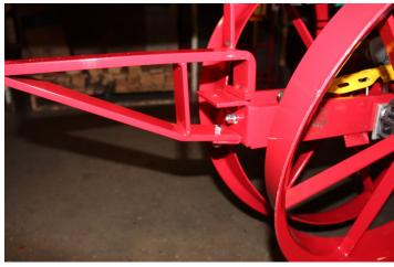
15) Re-install the wheel scraper assembly by removing one wheel scraper blade.
