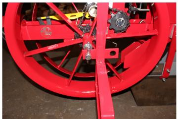
4) Install the plant stand onto the axle and re-install the cotter key as shown. Repeat on the other side.
