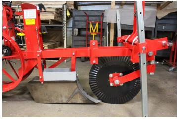
1) Install the hitch assembly onto the unit by using four  $\frac{1}{2}$  x 1  $\frac{1}{2}$  hex head bolts, lock washers and nuts.
