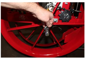
3) Install the plant stands by removing the outer cotter key from the axles.
