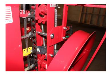
7) Install plant stand onto plate by using two  $\frac{3}{8}$  x 1 hex head bolts and flange nuts. Repeat on other side and tighten all fasteners.
