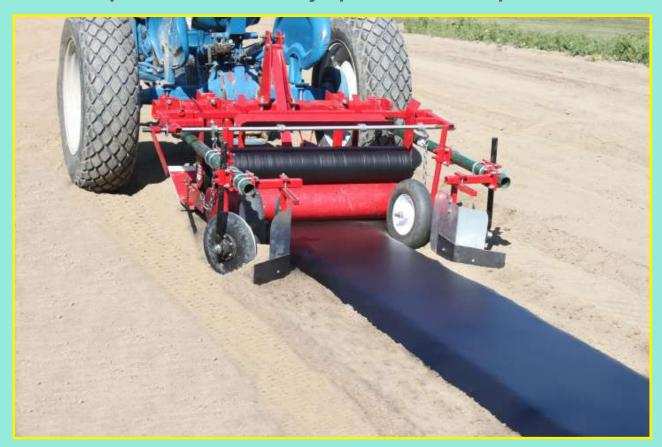
The Model 92 converts to a **Model 92B** Bed Shaper through implementation of deeper wings under the front leveling pan. Rear dirt shield and scrapers level the edges next to the plastic.
