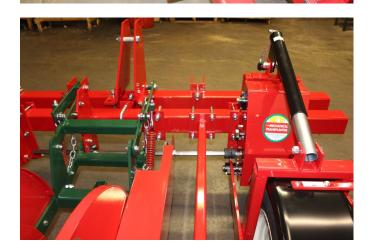
13) Install pipe stand and bracket to front bar by using two 5844 U-Bolts, lock washers and nuts.
