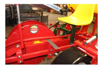
Install barrel mounts by using one 3444 U-Bolt, 2 Nuts and lock washers; ensuring 21" on center for barrel.
