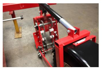
Lay out toolbar by marking row center and drive center. Mark A-frame drop locations using 26" centers for Cat I or 32" centers for Cat II hitches.
