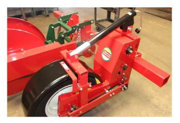
Install the other half of the hex coupler onto the drive and remove the guard.
