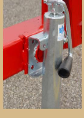
7. Bolt hitch to end of tongue using four 7/8 x 2" bolts and lock washers. Bolt hitch on as shown to plant on flat ground and flip hitch over to plant on beds.
