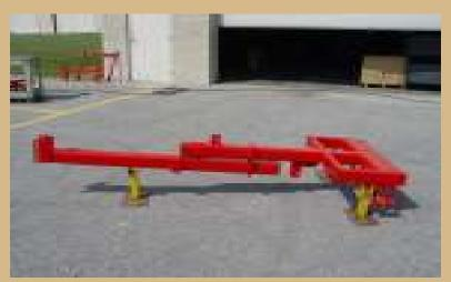
Place one 1/2 x 1" safety bolt in hole on back of tongue. Hold bolts in place with lock nuts. Set tongue length to allow clearance of tractor ties when turning.
