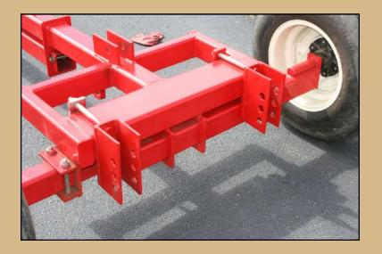
9. Install the lift assembly brackets to the main frame. These should be set 26-1/2" apart on center. Secure with 5/8" thick plates and 1 x 9-1/2" bolts, nuts and lock washers.
