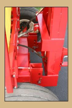
27. Attach lift assembly to brackets on main frame. Use the lower holes on the brackets and hold lift assembly in place using 1-1/8" pins and clip pins.
