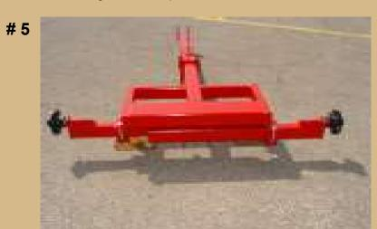
5. Slide both axles into square plates under main frame. Secure axles to frame with two 1/2 x 2-1/2 x 6" plates and four 3/4 x 6" bolts and lock washers (Photo #5A). To plant on flat ground, spindles must be up. To plant on beds or for higher trailer profile, spindles must be in down position. Measure and set wheel centers.
