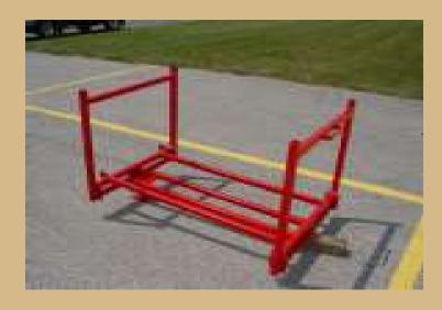
11. First assemble saddle frames by bolting arches with handles to saddle main frame end without booster block and arches without handles to end with booster block (Photo 14A). Use sixteen 3/8 x 1-1/4" bolts and lock nuts.
