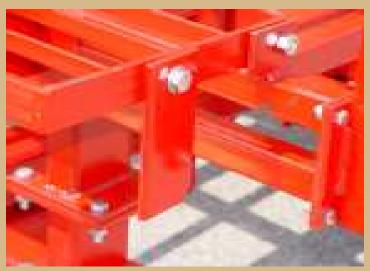
22. Insert #43 bushing into 2-1/2 x 6" step lock plate. Bolt plate to right side of right step using 1/2 x 1-1/2" bolt and lock nut. Tighten all step bolts. Raise step when planting so tractor tires do not hit on tight turns. (Photo 21A) shows step locking plate in the up or locked position.
