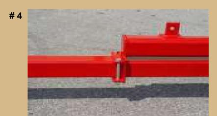
4. Secure tongue to main frame using 1/2 x 2 x 6" plate and two 5/8 x 6-1/2" bolts and lock washers.
