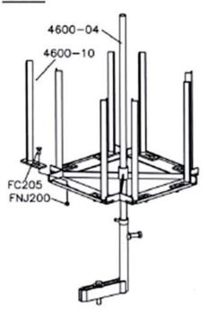
4600-04 Plastic Tray Pipe 4600-07 4 Place Bottom Tray 4600-10 Plastic Tray Holder Arm 4600-18 Carrousel Pipe 4600-19 Top Disc 4600-20 Top Spring Plate 4600-21 Back Spring Plate 5150 Carrousel Arm Carrousel Base 5152 6600-05 Carrousel Collar 6600-07 6 Place Bottom Tray 3/8x3/4" Carriage Bolt FC205 FF105 1/4x3/4" Flange Bolt 5/8x2" Hex Head Bolt FH431 FH443 5/8x3-1/2" Hex Head Bolt FHN331 1/2x1" Nylon Hex Head Bolt 5/8" Lock Washer FL400 FNJ200 3/8" Jam Nut 5/8" Flat Washer FW400
