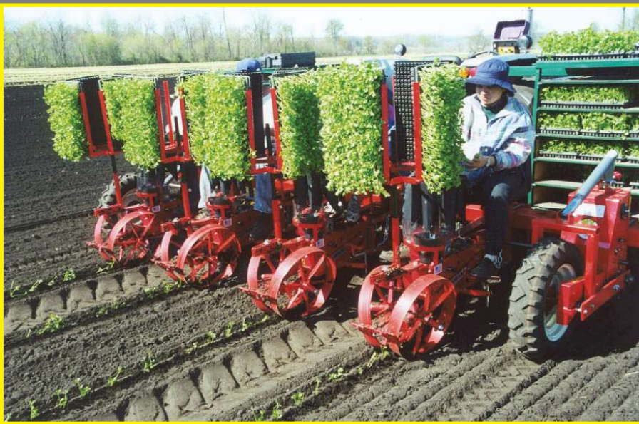
4-Row Model 5500W with EZ-17 gauge wheel drive system
