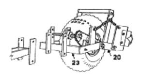
Run the float wheel with only 4 to 5 pounds of pressure during operation. Plant spacing can be changed slightly by increasing or decreasing the tire pressure.
