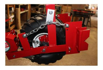
9. Install the drive clamps by using two 1/2 x 1 1/2 hex head bolts, two #43 bushings, lock washers and hex nuts.
