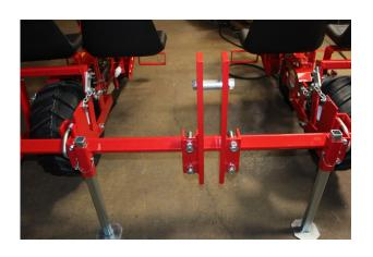
6. Install on toolbar by using two 7/8 U-Bolts, lock washers, and nuts. Center on toolbar and tighten.
