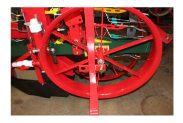
16. Install plant stand on the unit by sliding the lower plate onto the axle. Reinstall cotter pin and bend over longer leg to secure.
