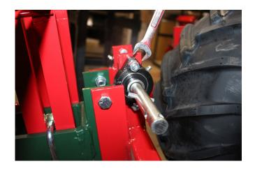
4.Install the inside chain guard by removing the outside 3/8 hex nut on the drive.
