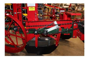
8. Install the outside chain guard and secure with two #17 clip pins.
