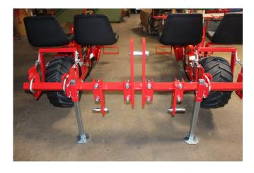
8. Install lower A-Frame drops on the toolbar, centering the hitch pin on the mark you made on the toolbar.
