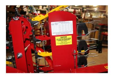
6. Refer to spacing chart on guide for desired plant spacing. IE - For 18" plant spacing you would use the following sprockets:
