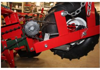
7B. Note for this spacing, you will need to add the extra links attached to the drive for it to fit properly.
