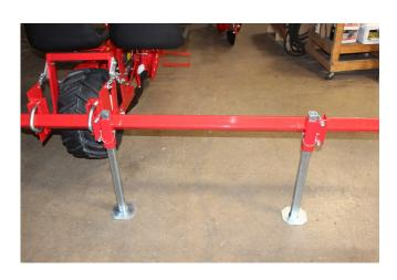
3. Install the parking stand brackets and stands by using two 726 U-bolts, lock washers and hex nuts. Leave enough room for the second unit you can slide next to it once you have the drive installed. Now your unit will stand on its own
