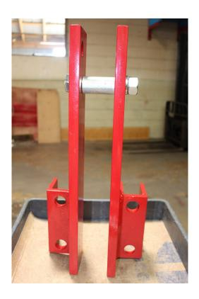
5. Assemble the A-frame uprights by using one 7/8 x 5 hex head bolt, spacer, lock washer and hex nut.
