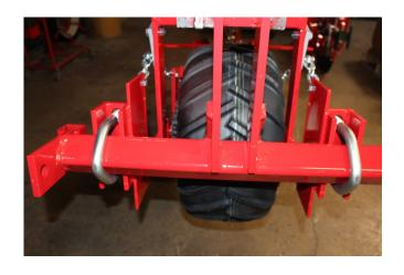
10. If using a single row hitch, secure the hitch with two 7/8 U-Bend, 740 U-Bolts, lock washers and nuts. Center the hitch by using the drive wheel as a reference point and tighten.
