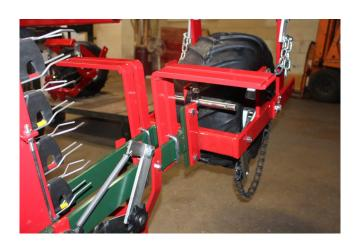
3. Install the seat bracket onto unit by using one 727 U-Bolt, flat washers, lock washers and hex nuts.
