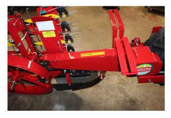
7A. Install the unit drive chain as shown.
