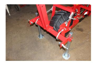
11. Install the hitch pins and pipe stands onto the hitch.
