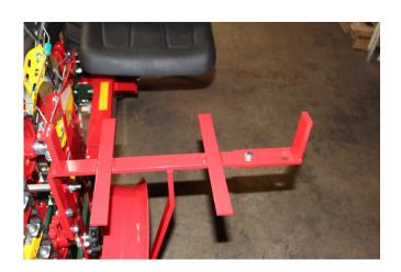
18. Install the adjustable plant box tub by using one 3/8 x 1 hex head bolt and serrated flange nut.
