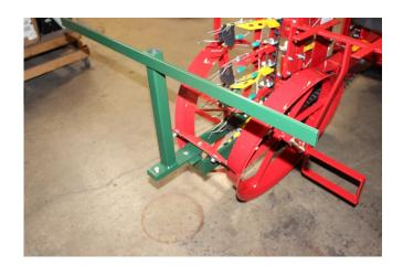
19. Install the rear shelving "T" by using one 3/8 x 1 1/4 hex head bolt, lock washer and nut.
