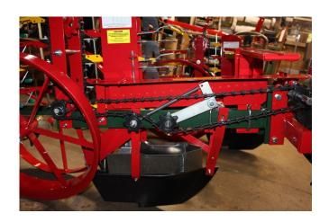
5. Re-install hex nut onto drive. Secure the other end of the guard by using one  $3/8 \times 1$  hex head bolt and nut, inserting it through the frame of the unit and guard.
