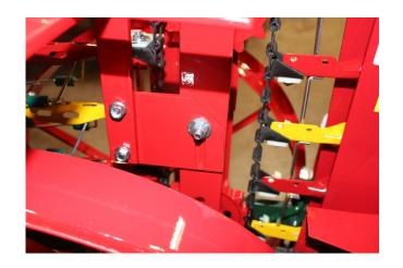
17. Install upper part of plant stand onto plate. Attach with two 3/8 x 1 hex head bolts and serrated flange nuts. Leave loose until you have both sides on, then tighten.
