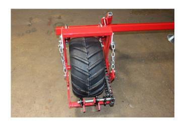
4. Install second drive onto tool bar. See set up for single row instructions.
