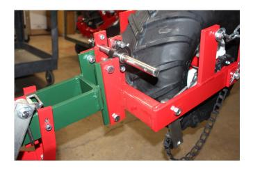
2. Remove the clip pin and sprocket package from drive
