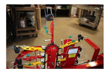
12. Install the extra pocket if needed by using a 7/16 wrench.
