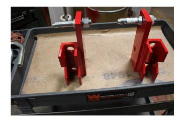
7. Install hitch pins into the A-frame drops using lower holes. The pins can be installed facing in or out of the bracket.
