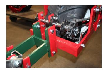
1. Install the drive system onto the unit by using four  $1/2 \times 1 \cdot 1/2$  hex head bolts, lock washers and nuts.
