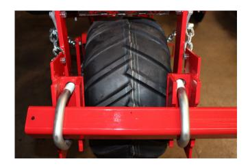
2. For this application we are turning the clamps to the inside to be able to fit on the toolbar. Align the mark made on the tool bar with the center of the drive wheel and tighten.
