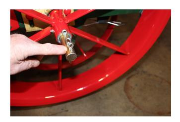
15. Remove the outer cotter pin on the packing wheel axle.
