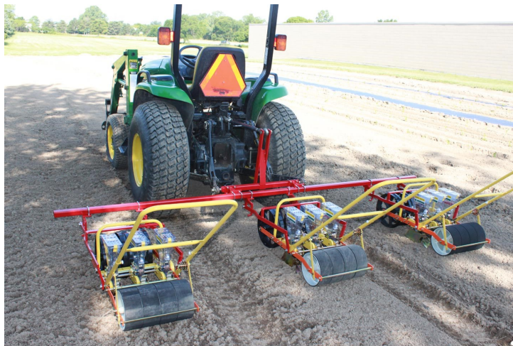
Multiple seeders may also be assembled on a longer toolbar to plant separate beds at a time
