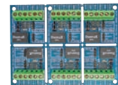
P/N - CM940B 6 Way Programmable Relay Card Can be separated into single relay cards. F.01U.275.899
