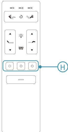
**NOTE:** To restore the preset buttons back to their original factory settings, hold **FLAT** and **ZERO-G®** simultaneously for at least 5 seconds. The original presets will be restored.
