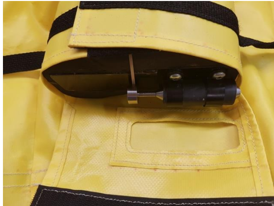
Figure 16: Activation mechanism aligned with opening in flap
