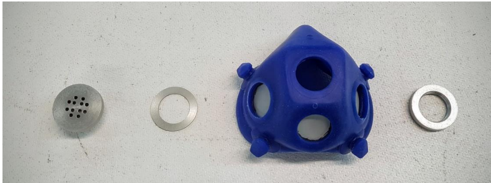
Figure 14: Nose cone assembly sorted from outermost to innermost components
