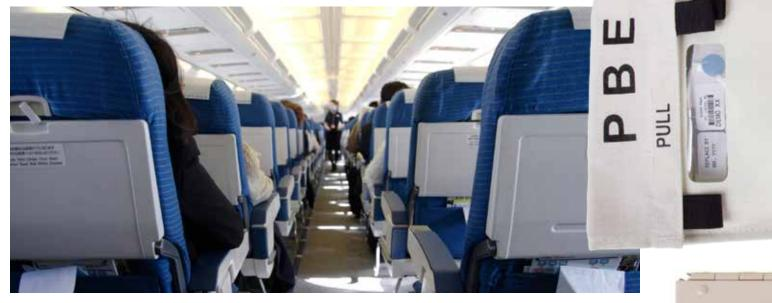
The Essex PBE is a lightweight, portable, self-contained, personal breathing device designed to safeguard flight attendants and crewmembers from the effects of smoke, carbon dioxide, harmful gases and oxygen deficiency while managing fire, smoke or fume emergencies. The equipment improves the wearer's visibility in smoke-filled compartments, protects the head and face from melting or dripping plastics, and shields the head against brief exposure to heat and flame.
