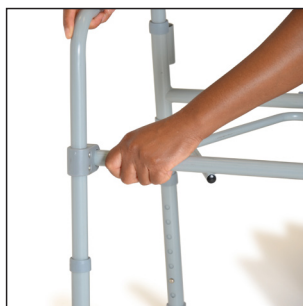
Insert the front cross bar into the front brackets (located on the front legs of the commode frame). Ensure both metal pins "CLICK" completely into holes
