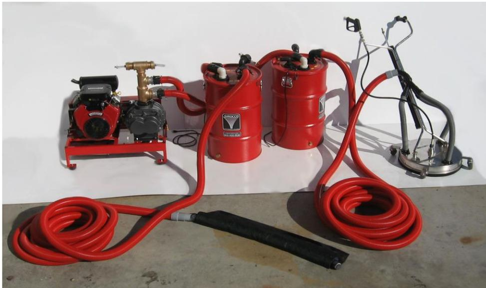
**Auto-pump-out in each tank is capable of up to 40 gpm against the vacuum!** and **each tank has dual inlets!**
