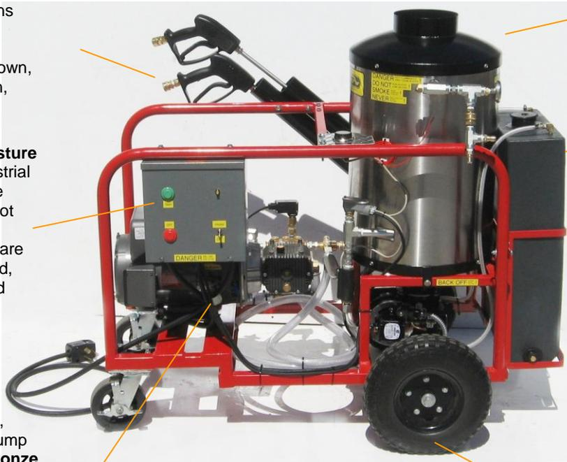
High efficiency Coil-tank assemblies include stainless steel shell, double insulated base, Redundant temp. controls,
