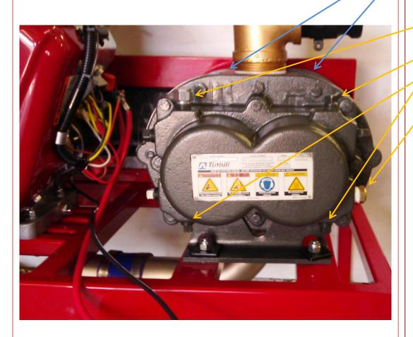
Grease fittings for the rear (drive-end) of the blower are located at the back, next to the pulley, just in front of the beltguard.
