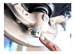
Repeat these steps to the other side of the vehicle. Place the vehicle down on its own weight and adjust the lower arm alignment cams to the marks you made during step 2. Torque the alignment cam nut to factory specifications (First pass: 133 ft lbs. Second pass: 90-105 degrees) Inspect your work and then have the final alignment set by a qualified shop.
