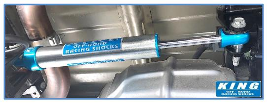
**DOUBLE CHECK ALL HARDWARE:** Make sure the shock is installed properly and all hardware is tight. Recheck all hardware after 100 miles and periodically after that as part of routine maintenance.
