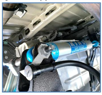
3. Place the shaft end in the mount on the crossmember, install the original bolt and tighten to factory specs.
