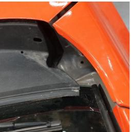
2. Prop open your hood and start on the driver side hood hinge with the (2) 12mm nuts, mark the hood and hinge to ensure the hood is still aligned correctly after install. Loosen both nuts enough to be able to slide in the mount underneath.
