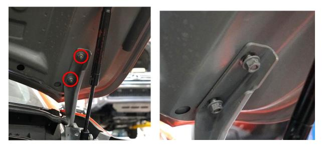
**3.** Starting with the front slot, slide the A-pillar in place and position the mount forward so the notch is sitting over the hood, now make note of where the mount sits on the hood and move the mount enough to apply your edge trim to the edge of the hood.
