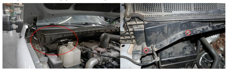
**3.** Thread the provided (2) M6 Hex Bolts and M6 washers into the holes. On the other end of the bolt install the remaining (2) M6 washers and (2) M6 Nylock nuts. Have the (2) bolts tightened by hand leaving room for the mount. Slide the SDHQ Power Module Mount in between the plastic cowl and M6 washers as shown. Now completely tighten the M6 bolts using a 10mm socket and wrench.
