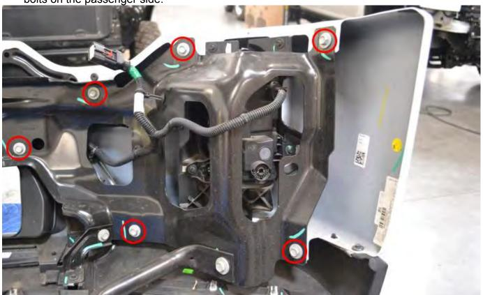
**4.** Uninstall the (3) 14mm bolts on the driver and passenger factory fog lights. If your vehicle did not come with Factory Fog Lights, remove the faux Fog Light Bezel and install the replacement Bezel/Trim Ring before proceeding.
