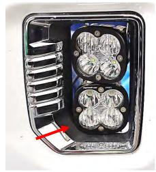
7. Install SDHQ Fog Light Mount onto bumper using the 14mm factory bolts loosen the bottom two bolts as necessary. Repeat for the passenger side fog light mount.
