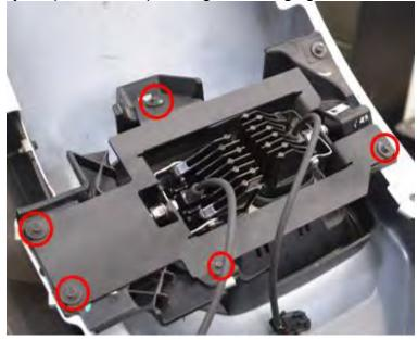
**8.** Reinstall factory bumper mounting brackets on the driver and passenger side using the same 14mm factory bolts that were removed. Tighten all (12) 14mm bolts and give the lights and bumper an overall look to ensure it is how you want it, make adjustments as necessary.
