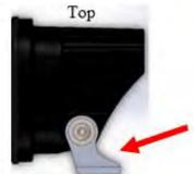
**6.** <u>Installing the lights.</u> First, mount the Top light in the SDHQ Fog Light Mount upside down. The bottom mount will slide in the lower slot after. Do NOT tighten the Baja Design Brackets down in the SDHQ Fog Light Mount until desired angles are set up. It is optional to trim the black plastic bezel to help fitment as shown below.
