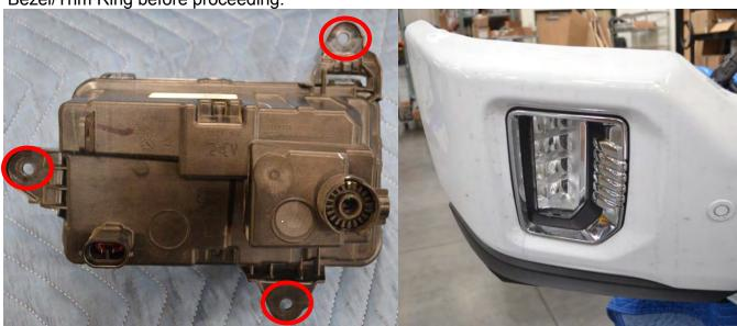
**5.** <u>Preparing the lights.</u> Open the Baja Design Squadron Kit and prepare the lights for install. Do not install the SDHQ Fog Light Mounts into the bumper until all lights are installed into the mounts. Refer to the Baja Design instructions as necessary, orientate the Baja Design brackets as shown below.
