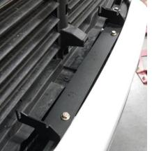
7. Install your Light Bar. Use a body saw trim the lower center grill mount to fit the profile of the light bar if required. Check fitment by placing the light bar into the mount and remove more material as needed using a dremel with a barrel sander attachment. Place the ¼" washers on the between the mount and light bar when running Onx6 Light Bars.
