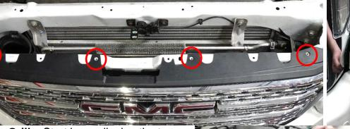
4. Removing the Grille. Start by unclipping the top edge of the grille as shown. Then carefully pull out the bumper from the driver side popping all (8) clips holding it to the vehicle. The front fender panels will need to be lifted to allow the grille to slide out from behind. When removing the passenger side of the grille the front camera wire will need to be disconnected shown below in blue.
