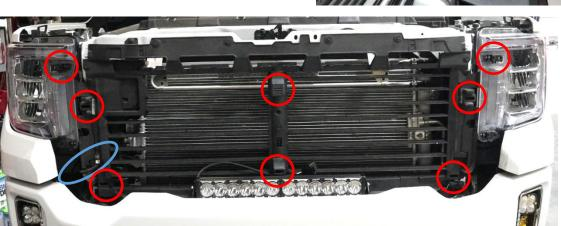
For questions or help with the installation, please call SDHQ Offroad @ 480-633-2929 Mon.–Fri. 8:00am–5:30pm and Sat. 8:00am–3:30pm Arizona Time. www.sdhqoffroad.com Page 4 of 6 5. Cutting the Grille. Use a pair of flush cuts to start the vertical cuts. Use a body saw to finish cutting the piece away from the grille. Do not remove the bottom clip, in blue, when cutting.
