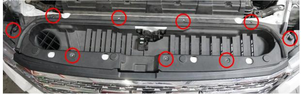
**3.** Prepping the Grille. Remove the (4) 10mm bolts on top of the grille, circled below in red. Next, the front fender panels will need to be partially removed by pulling the front clip free but leaving the panel attached as shown below. Repeat process for both sides.
