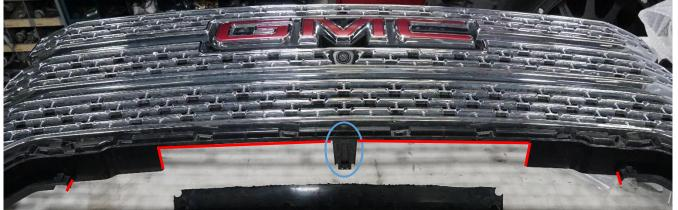
6. Slide the supplied (2) 3/8" Clip-On Nuts on to the bumper as shown below. Place the mount on top aligning the holes and loosely thread in the (2) 3/8" bolts supplied with your light bar.
