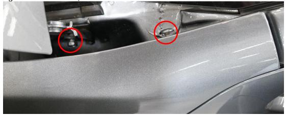
**5.** Position the driver side support bracket as shown. Thread (1) M6 bolt and (1) ½" washer into the threaded hole to secure the support bracket.
