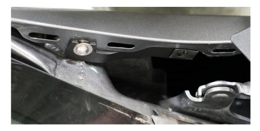
**6.** Carefully lower the driver side mount between the hood hinge and fender. Once lowered, insert (1) M8 bolt and (1) 5/16" washer through the lower mounting hole. Place (1) aluminum spacer between the mount and the hood hinge. Begin threading the M8 bolt. Align the driver mount and support bracket, and thread (1) 1/4" bolt and washer into the support bracket.
