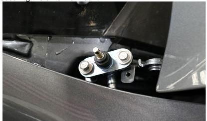
4. Starting on the driver side, remove the 13mm head bolt and Torx T30 head bolt circled below.
