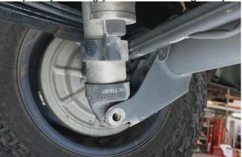
**3.** Align the shock guard onto the lower mount and replace the shock bolt with the supplied M12 flange head bolt and nut. Leave the bolt loose to allow the shock guard to be adjusted.
