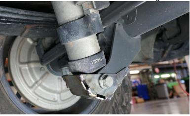
**4.** Next swing the shock guard up so that it aligns the slot on the shock mount. Slide a capture plate in the slot and align it with the hole on the back of the shock guard. Using the supplied 3/8" bolt, fix the shock guard to the rear of the mount leaving the bolt loose for now.
