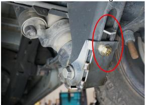
**5.** Repeat steps 2-4 for the other shock and tighten all 3/8" hardware. Lower the vehicle down to ride height and tighten the lower shock bolts to factory torque specs. Enjoy your new SDHQ Built Chevy/GMC Raer Shock Guards!
