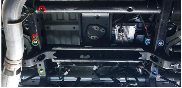
5. Using a jack or other method of lifting the Air Compressor Mount Assembly, position the assembly onto the frame by sliding the driver side of the mount in between the frame and loosened bolts from Step 4. Thread in the passenger side frame bolts, then tighten the frame bolts to secure the Air Compressor Mount to the frame. Finish wiring and plumbing your Air System. Replace the exhaust heat shield and bolts. Enjoy your new Air System!
