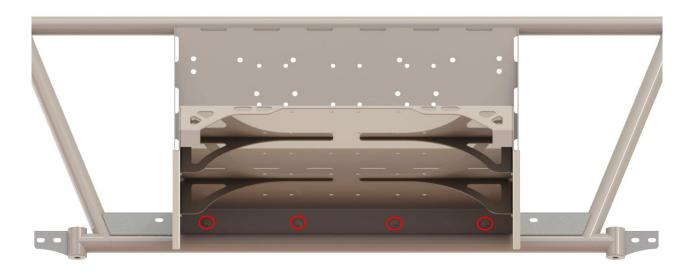
3. Align the Driver Side Plate next to the Front Plate and Floor Plate. There is a total of (7) 5/16" – 18 x ¾" Grade 8 Hex head bolts that will be used on this side. (3) bolts will connect the Driver Side Plate and the Front Plate. The other (4) bolts will connect the Driver Side Plate and the Floor Plate. Be sure to use the 5/16" washers on both sides of the bolt.
