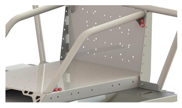
**6.** Use (2) 5/16" – 18 x 3/4" Grade 8 Hex head bolts, (4) 5/16" washers and (2) 5/16 – 18 Lock Nuts for each tie down mount. Bolt the mounts as pictured below. The mounts can be placed where needed on the Bed rack.
