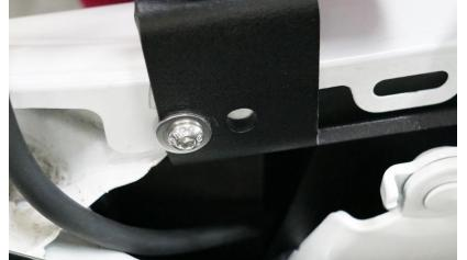
8. Repeat Steps 4-7 for the passenger side. Once the mount is tight, tighten the (2) 10mm head bolts securing the antenna mount to the truck. Proceed to Step 11.
