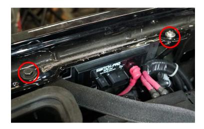
6. Reinstall the passenger side hood trim. Use the supplied zip tie to secure wiring once complete.
