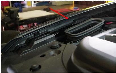
4. With the hood trim removed, remove the factory bolt circled below using a 13mm socket.
