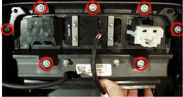
**4. Mounting the Switch Pros Keypad.** Put the Switch Pros Keypad through the back of the SDHQ provided panel. Flip the assembly over and thread the (4) Switch Pros provided studs into the back of the Switch Pros Keypad by hand. Do not over tighten as the keypad is prone to stripping. Place the (2) Switch Pros Provided backing reinforcements over the studs and tighten the (4) Switch Pros provided nuts by hand with an 8mm socket.
