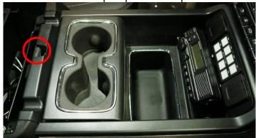
3. Unscrew the (7) bolts circled in red holding the panel in place with the T20 Torx. Remove the 120v and USB ports (if equipped) from the factory panel. Do so by compressing the clips and pushing out towards the front of the panel. Install them in the new SDHQ provided panel. If 12
