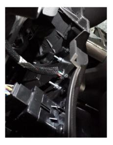
**11.**Reinstall the Instrument Panel Knee Bolster, attach the electrical connectors and push panel into place until clips snap in. Reinstall the Hood Release if removed and the (5) 10mm bolts.
