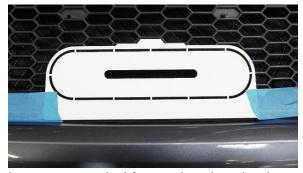
onto the bumper and remove the bumper to cut. A body saw is recommended for cutting the plastic.
