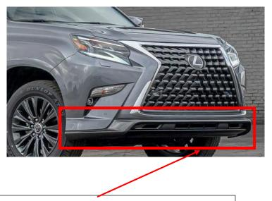
If you have a 2020+ GX460 with the "Sport Design Package" the removal of the extra aero that comes in the package will leave several holes that will not get cut off when trimming the bumper. Use The supplied 3/8" Push-In Rivets to plug the holes
