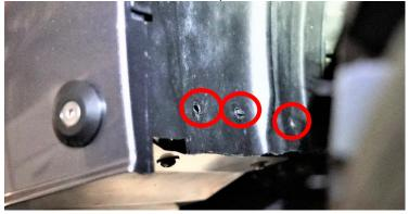
**13.** Now that the fender liners are trimmed, pull the Fender Liner Brackets out and place Clip-on nuts over the remainder of the holes. Then replace the Fender Liner Bracket and bolt into place on Skid Plate. Next you will use the remaining delrin body washers and counter sunk ½"-20 bolts and bolt the fender liners to the Fender Liner Bracket.
