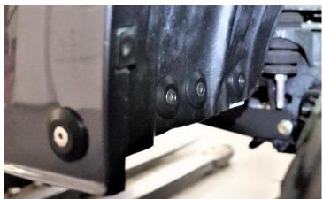
**14.** Use the provided ½" bolts, washers, and lock nuts to mounts the bottom of the bumper to the bumper bracket. Check to be sure all hardware is tight and reassemble the rest of your vehicle reversing Steps 3 – 1 in the 4Runner Hidden Winch Mount Install Instructions, 54-1650-G5. Enjoy your **SDHQ Built Skid Plate System** for your 2014-Current Lexus GX460!
