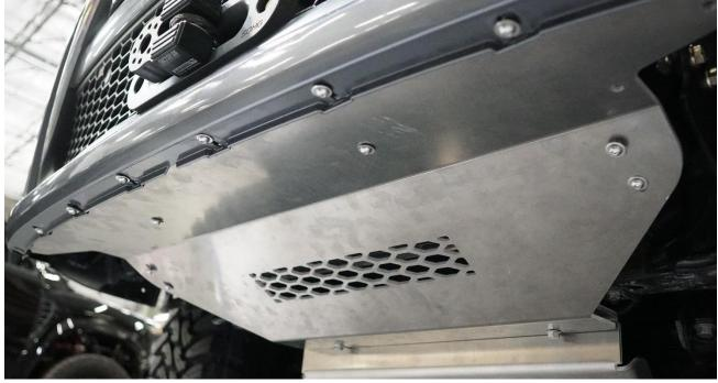
9. Mount Skid Plate Backers. Take the Driver and passenger Skid Plate Backers and install them with 1/4"-20 hardware as shown below, the outermost bolt will go through the bumper like the Main Skid Plate. Then place the (3) Clipon nuts per side once the backer is tight.
