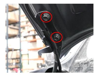
3. Remove the rear bolt and rotate the mount to align with its hole. Insert bolt through the rear hole of the mount and thread into the hood. Tighten down bolts while aligning hinge with paint outline of previous location on the hood. On the passenger side a small clip will need to be removed to access the rear bolt.
