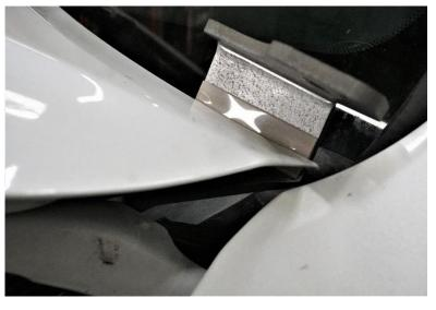
4. Repeat Steps 2-3 for the Passenger Side, while first unclipping the windshield washer hose from the hood hinge, the mount goes between the washer hose and hood hinge when installed. Reinstall Washer hose clip when finished.
