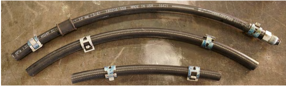
Hoses with factory clamps installed.
