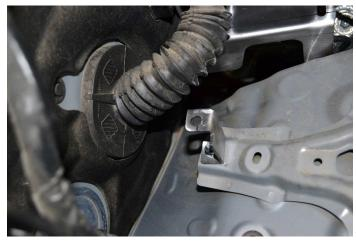
Threaded Rod available such that the battery can still be secured into the Main Battery Mount.
