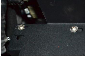
M8 Nylock Nuts and the (2) M6 S.S. Button Head Flange Bolts. Be sure the Flange Nuts on the Threaded Rods are secure as well.
