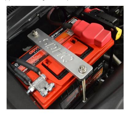
**14.** With the battery in place, the install of the SDHQ Dual Battery Kit is complete. Now, the battery will need to be wired. If the SDHQ Dual Battery Wiring Kit (SDHQ-50-3002-U1) was purchased, begin those Install Instructions.
