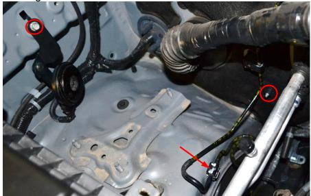
3. Installing the Dual Battery Kit. Slide the Vertical Support in between the loosened brake clamp and align the rear of the bracket onto the stud protruding from the firewall. Loosely tighten (1) M6 S.S. Nylock nut and (1) 1/4" S.S. Washer onto the stud protruding from the firewall. Loosely tighten the factory brake line bolt.
