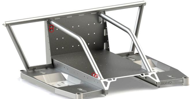
**6.** Use (2) 5/16" − 18 x <sup>3</sup>⁄<sub>4</sub>" Grade 8 Hex head bolts, (4) 5/16" washers and (2) 5/16 − 18 Lock Nuts for each tie down mount. Bolt the mounts as pictured below. The mounts can be placed where needed on the Bed rack.
