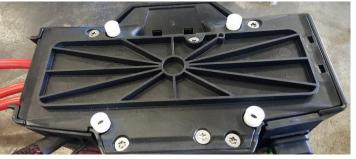
7. Mount your control box to the truck with (1)  $\frac{1}{4}$ " bolt, (2) washers and (1) lock nut, leaving the front 2 open until you are ready to install your bumper skin. Place the Control Box Mounting Bracket with the nutclips as shown below. Use the factory press in clip to hold the bracket in place.
