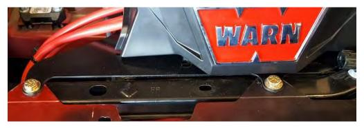
**17.** Plug your fog lights in. Reinstall the grille by clipping the bottom back in and reinstalling the upper 2 screws and 2 clips.
