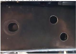
**10.** You can now install both of your Lower Support Brackets using the provided 7/16" hardware for the top, and the M12 bolts, washers, and nuts for the bottom. The passenger side will re-use 2 of the factory bolts and 1 of the new provided bolts. The driver's side will use all new provided hardware.
