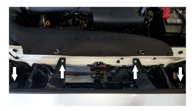
**2. Removing the factory front bumper.** Partially remove the front part of the inner fender well so you can get to the clips holding the outside of the bumper on. This is held in place by (2) 10mm
