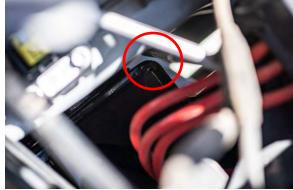
**9.** Temporarily install the driver's side lower support bracket to the winch mount. Use the slotted holes in the bracket to make your center marks in order to drill. Remove the factory box insert and discard. Drill the (2) 9/16" holes and deburr.
