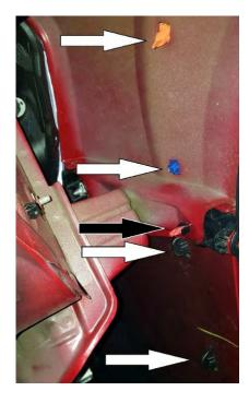
**3.** Remove the bumper skin from bumper mount by removing the 6 remaining clips located under the grille, and the 2 10mm screws on the bottom. Unplug the fog light harness and unclip it from the sheet metal.
