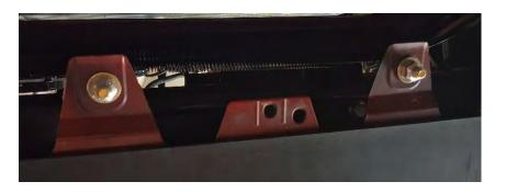
**16.** Loosely place the black factory outer plastic, with the Hawse cut out, onto the factory bumper skin. Adjust the Hawse so that it is lined up with your cut out. Pull the black plastic back off so you can tighten the Hawse. While the black plastic is still off, install the (2) ½ bolts and washers through the front of the Control Box Relocation Bracket to the Control Box Mounting Bracket. Now the front black plastic can be reinstalled with the factory clips.
