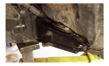
2. Place the Body Mount Cut Template against the body mount, centering the hole with the bolt as pictured. Sharpie around the template to mark what is needed to be cut. Use a Sawzall and the metal blade to cut the flat parts of the body mount. Use the grinder to finish cutting the body mount and clean up the cuts.
