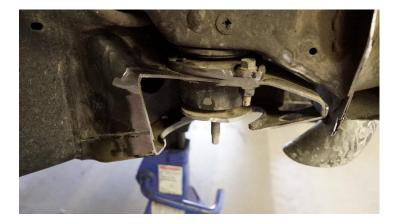
**3.** Verify fitment of the body mount plate. If the plate sits flush against the chopped body mount, tack it in place. If it does not, cut what needs to be trimmed. Once tacked in place, verify placement one last time and then weld it in place. Paint over any bare metal once complete to prevent any rust.
