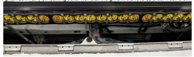
**6.** There is minor trimming that needs to be done to the TRD Pro Grille if you are using the top slot on the mount. Cut out the template below to the right. Place the only corner on the supplied template in the green circle pictured below. Mark the circle to be cut. Use a ¾" hole saw to cut into the grille. Repeat on the other side of the grille.
