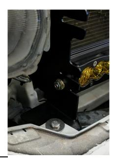
**5.** Install your light bar in the appropriate slot. Align the middle of the light bar to the bolt in the middle of the bumper. Repeat this step if you have more light bars going into the mount. Tighten down all (4) mounting bolts. Reinstall the grille in the reverse order it came off.
