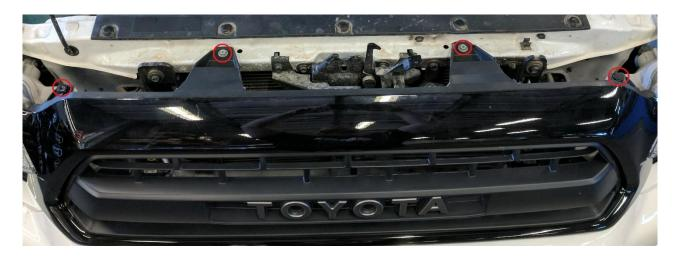
**2.** Gently pull the grille out towards the front of the truck. There are tabs in the top corners of the grille and along the bottom of the grille connecting it to the bumper. Set the grille aside for now.
