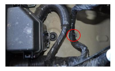
**3.** Place one ½" loom clamp on each run of wire pictured below. Place the 3/16" x ¾" Fender washer over the #10-24 x 7/8" S.S. Button Head Bolt. In the wheel well, locate the hole from the zip tie that was removed in Step 4. Place the S.S. Bolt and washer through that hole. Align the loom clamps over the bolt and use the #10-24 lock nut to secure the wires out of the way of the Power Module Mount.
