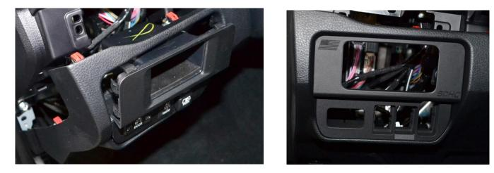
6. Installing the Switch Pros Keypad. For the Switch Pros Keypad, apply medium strength thread locker to the (4) #6 mounting studs and thread in by hand. Insert the Switch Pro Keypad onto the front of the panel. Place the backer spacer and then the backer on the back side of the cubby panel. The backer will be a tight fit and the SDHQ logo will be facing you when looking at it from the backside.
