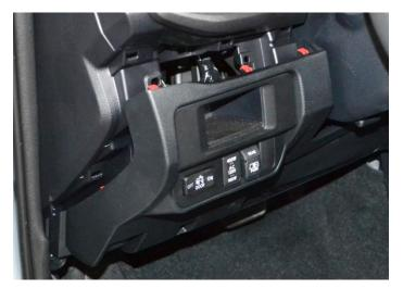
5. Disconnect the wires from the switches. Remove the cubby panel by detaching the (11) clips that secure the panel. The cubby panel pushes out the front of the panel as pictured. The switches need to be removed and installed in the new SDHQ cubby panel. Install the new SDHQ cubby panel into the dash panel.
