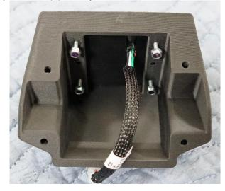
**10.** The ¾" hole in the center is for the Switch Pros wire to go through. Insert the (4) #10 socket head bolts through the bottom of the 3D printed mount. Secure the mount on the back of the panel with #10 washers and nylock nuts. Shown below with the SDHQ 9100 Mount.
