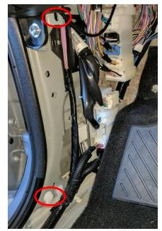
3. Next, the dash panel under the steering wheel needs to be removed. Using a 10mm socket, remove the (3) bolts at the bottom of the dash circled below in red.
