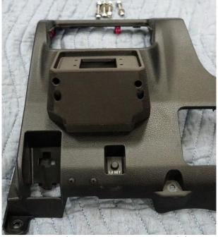
7. With the position for each hole located, use a drill with a 5/32" drill bit to drill the (4) mounting holes out. Using the dremel, clear out the material on the back of the panel as shown below.
