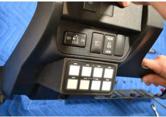
**11.** Finish wiring the Switch Pros Keypad and then reinstall the dash panel, kick panel, door sill trim, and floor mat. Enjoy your SDHQ Built Switch pro keypad mount!
