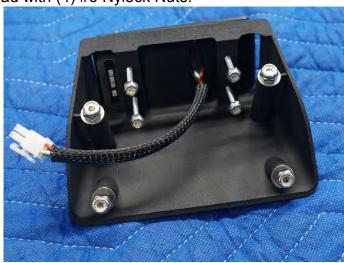
**10.** The ¾" hole in the center is for the Switch Pros wire to go through. Insert the (4) #10 socket head bolts through the bottom of the 3D printed mount. Secure the mount on the back of the panel with #10 washers and nylock nuts.
