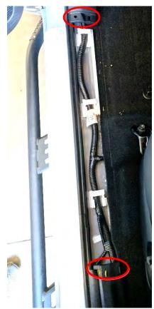
2. Remove the driver side kick panel. The kick panel has a plastic nut connecting the back of it to the fire wall. This can be unscrewed by hand. There is two clips connecting the panel to the truck by the door. Both clips pull back and out to the side at a 45° angle. If one or both of the white clips stay in the sheet metal, like the lower clip in the picture, it will need to be removed and reinstalled in the kick panel for proper re-installation.
