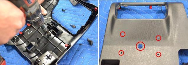
9. Installing the Switch Pros Keypad. For the Switch Pros Keypad, apply medium strength thread locker to the (4) #6 mounting studs and thread in by hand. Insert the Switch Pro Keypad onto the front of the panel. Secure the keypad with (4) #6 Nylock Nuts.
