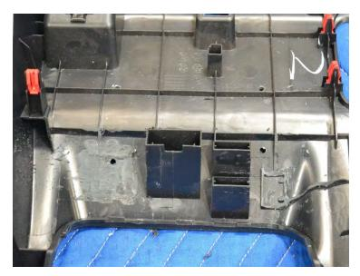
**8.** In the middle of the (4) holes, use a  $\frac{3}{4}$ " drill bit and drill a hole through the panel. If you do not have a big enough bit, use the dremel and cut a  $\frac{3}{4}$ " square out.
