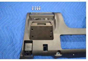
7. With the position for each hole located, use a drill with a 5/32" bit to drill the (4) mounting holes out. Using the dremel, clear out the material on the back of the panel as shown below.
