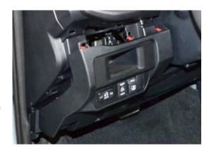
**6.** Line up the 3D Printed switch pro keypad mount and center it under the switches. When it is in the desired position use a 5/32" drill bit or another sharp slim tool to mark where the holes go.
